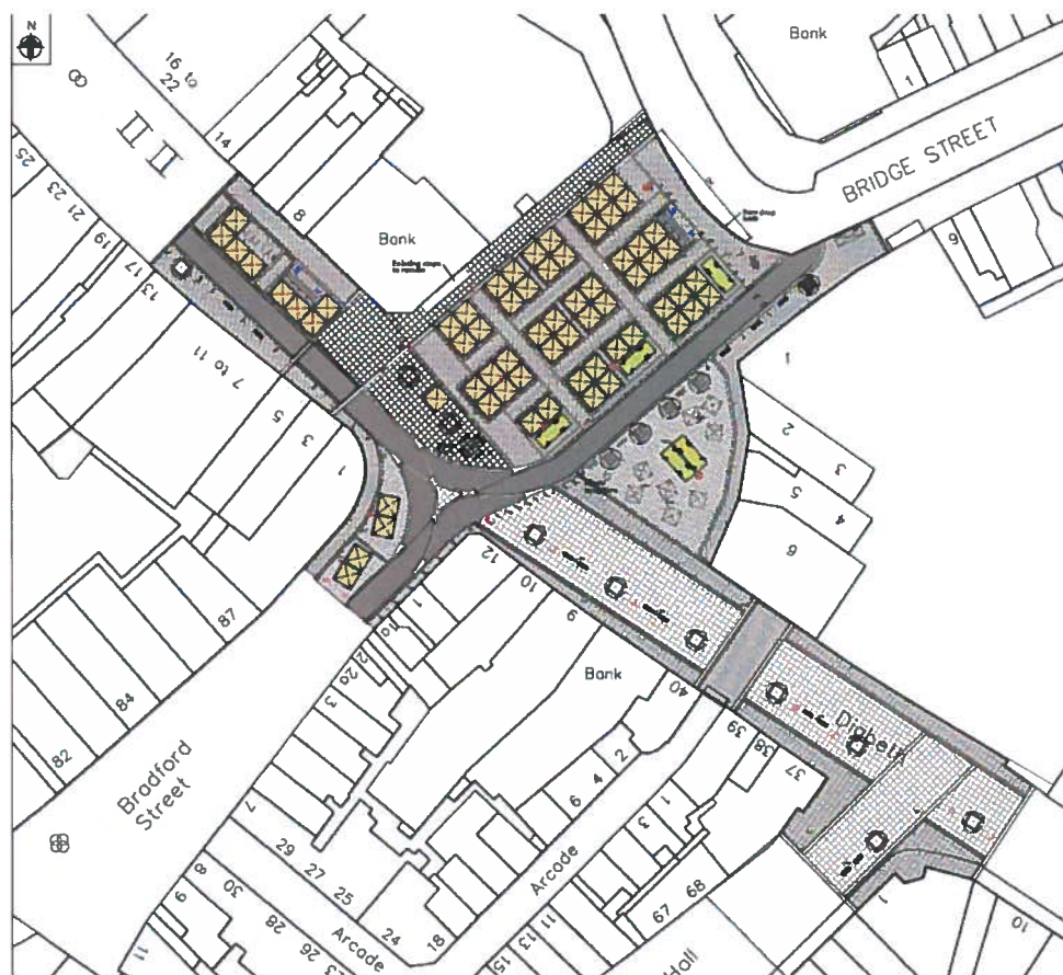
Figure 11 - Proposed Phase Two market layout after consultation - maximum stall number using 3x3 stalls. Refer to drawing ARP-PL-020.
