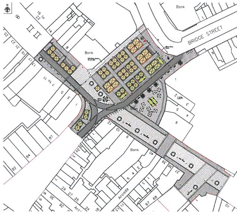
Figure 12 - Proposed Phase Two market layout after consultation - maximum stall number using mixture of 3x3m and 3x4.5m stalls. Refer to drawing ARP-PL-021.
