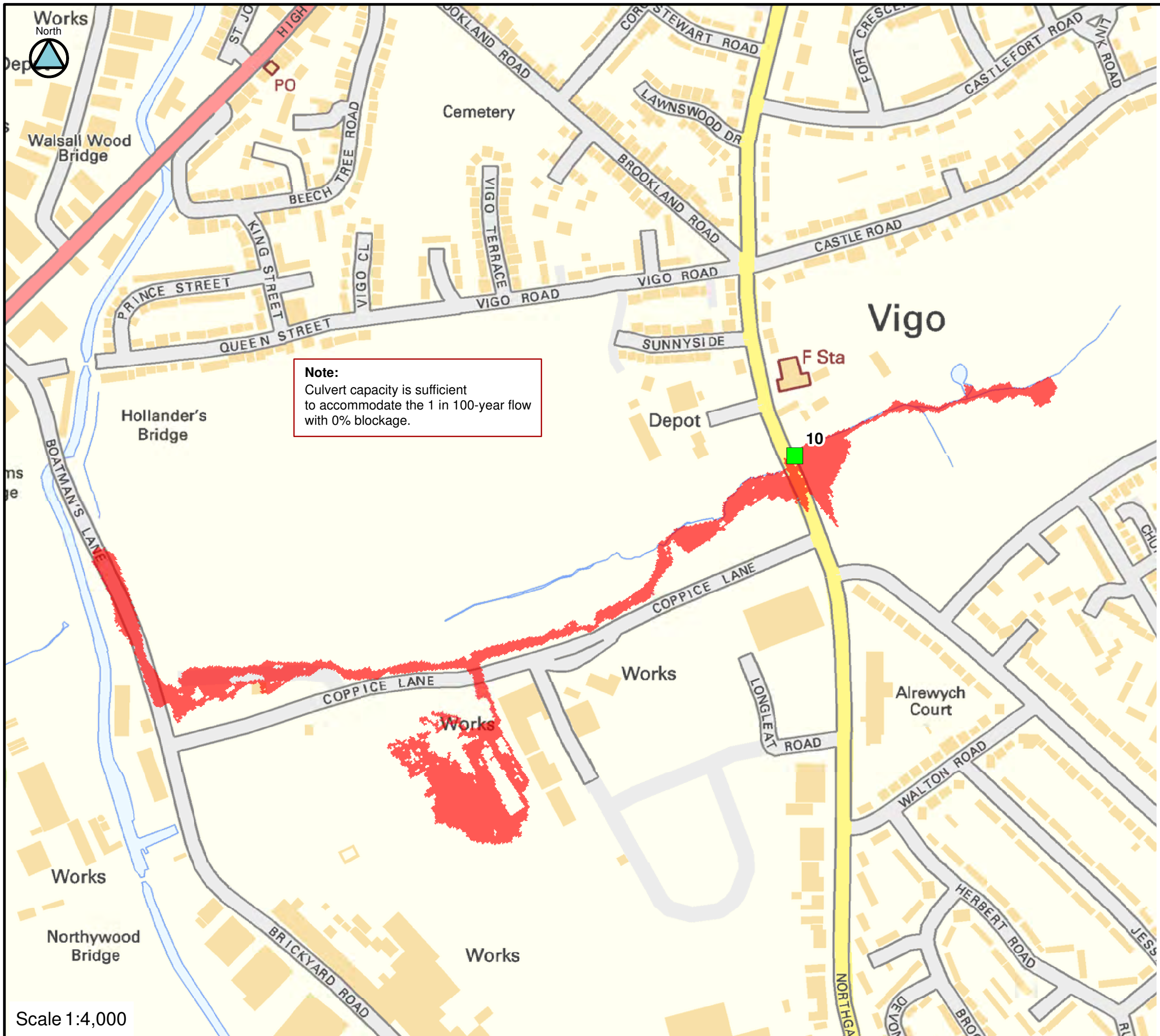
FIGURE C10-100-90 CULVERT 10 BLOCKAGE 1 IN 100-YEAR FLOOD EXTENTS
