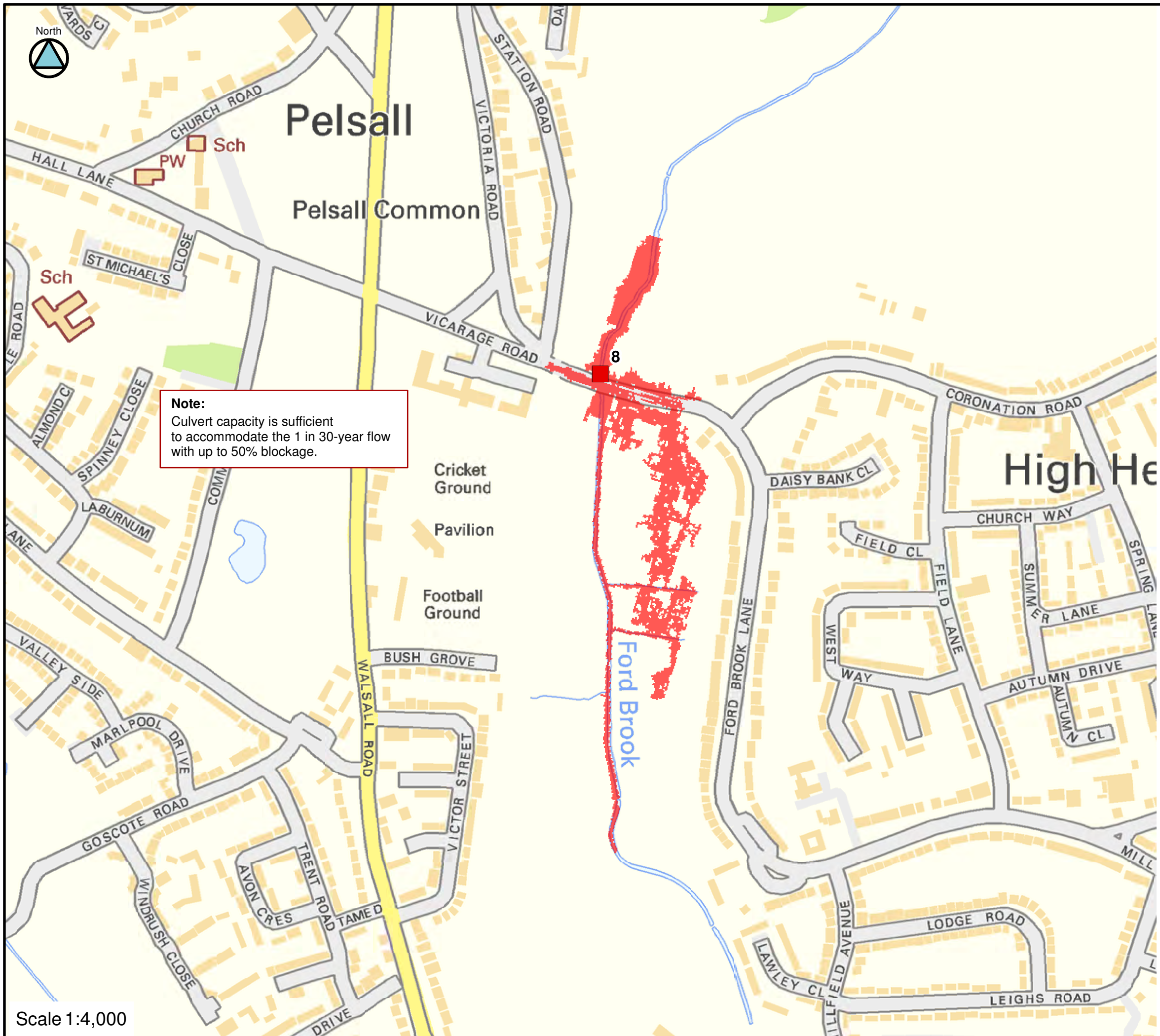
FIGURE C08-30-90 CULVERT 8 BLOCKAGE 1 IN 30-YEAR FLOOD EXTENTS
