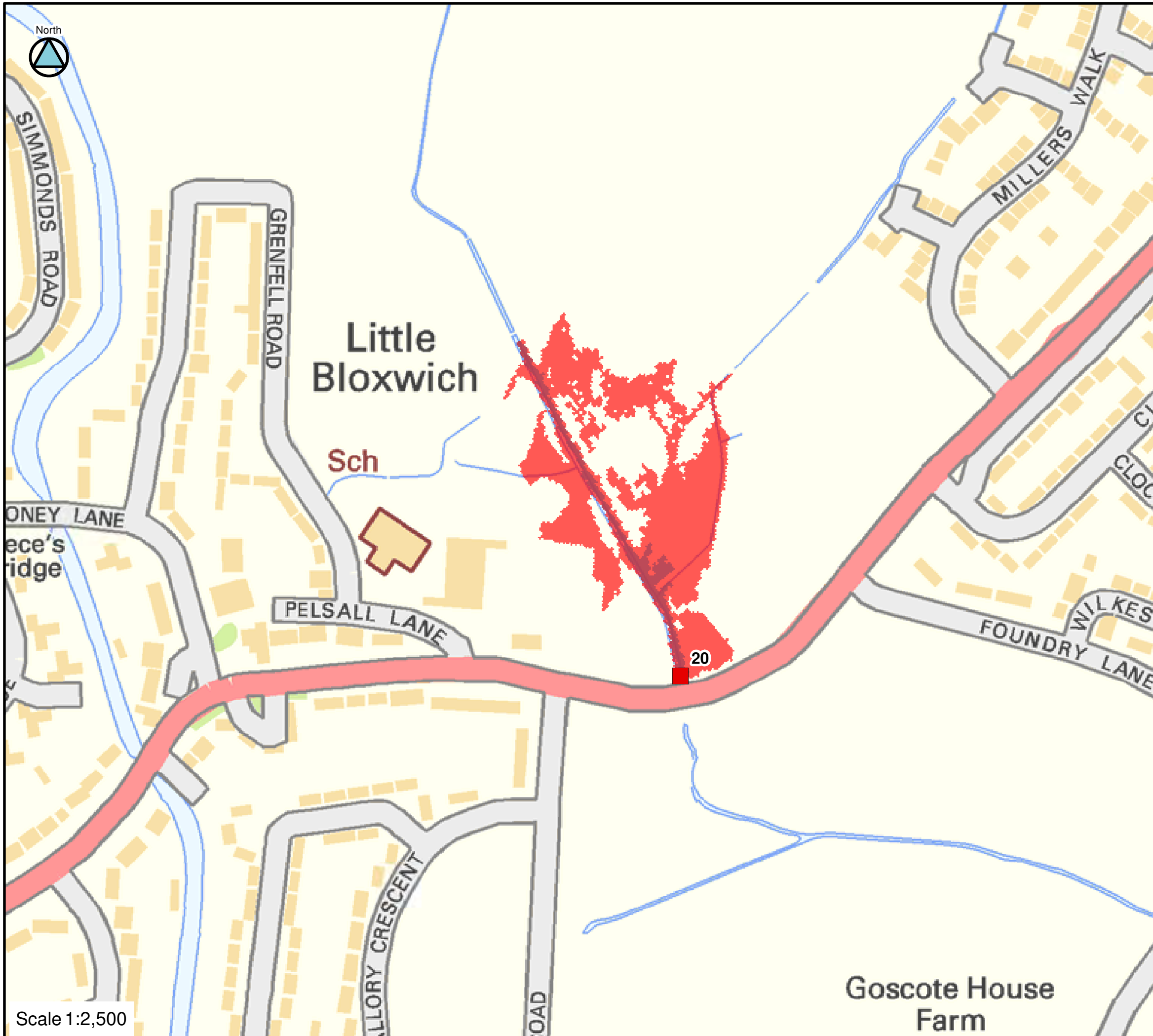
FIGURE C20-30-75 CULVERT 20 BLOCKAGE 1 IN 30-YEAR FLOOD EXTENTS
