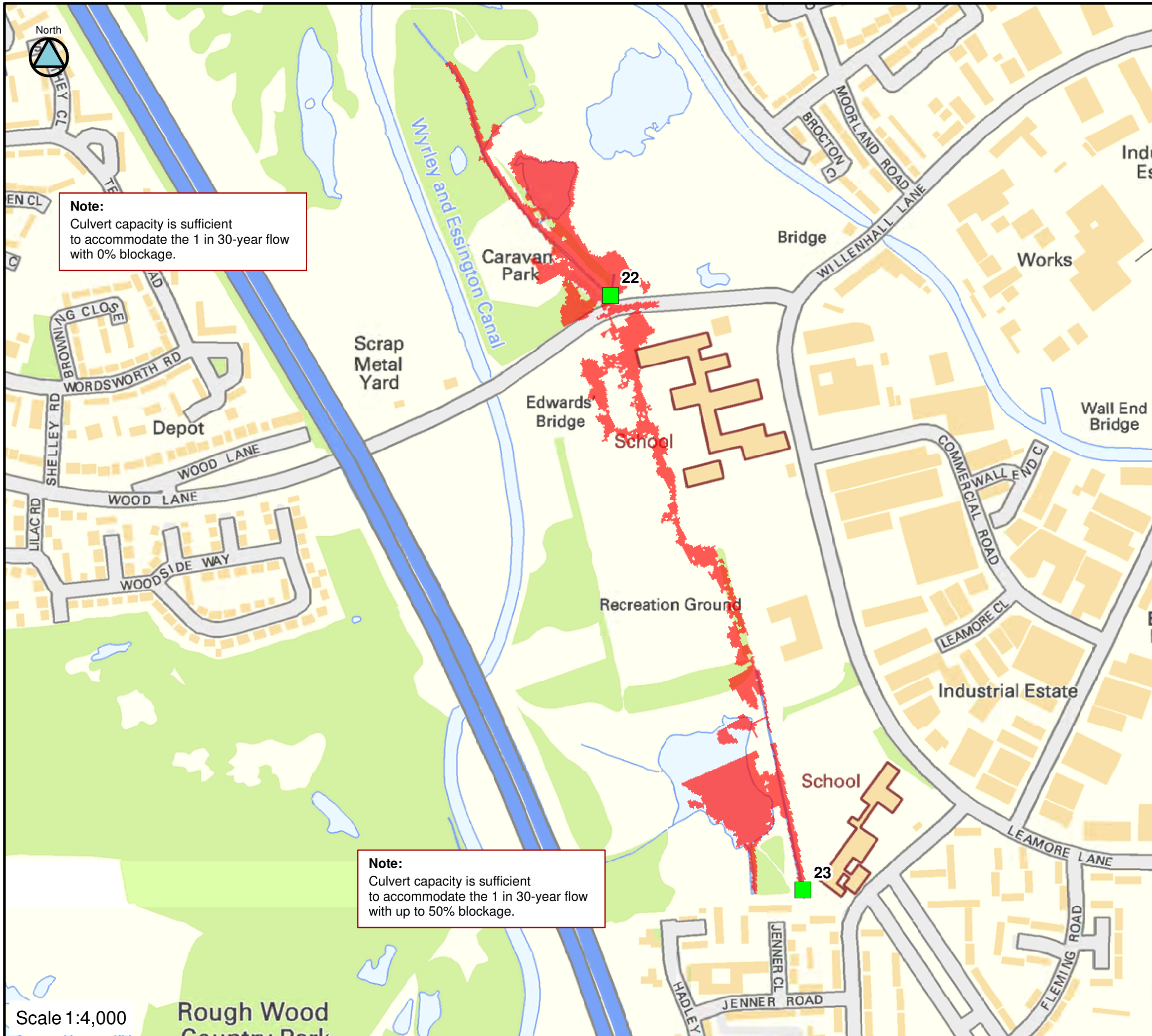
FIGURE C22-30-75 CULVERT 22&23 BLOCKAGE 1 IN 30-YEAR FLOOD EXTENTS
