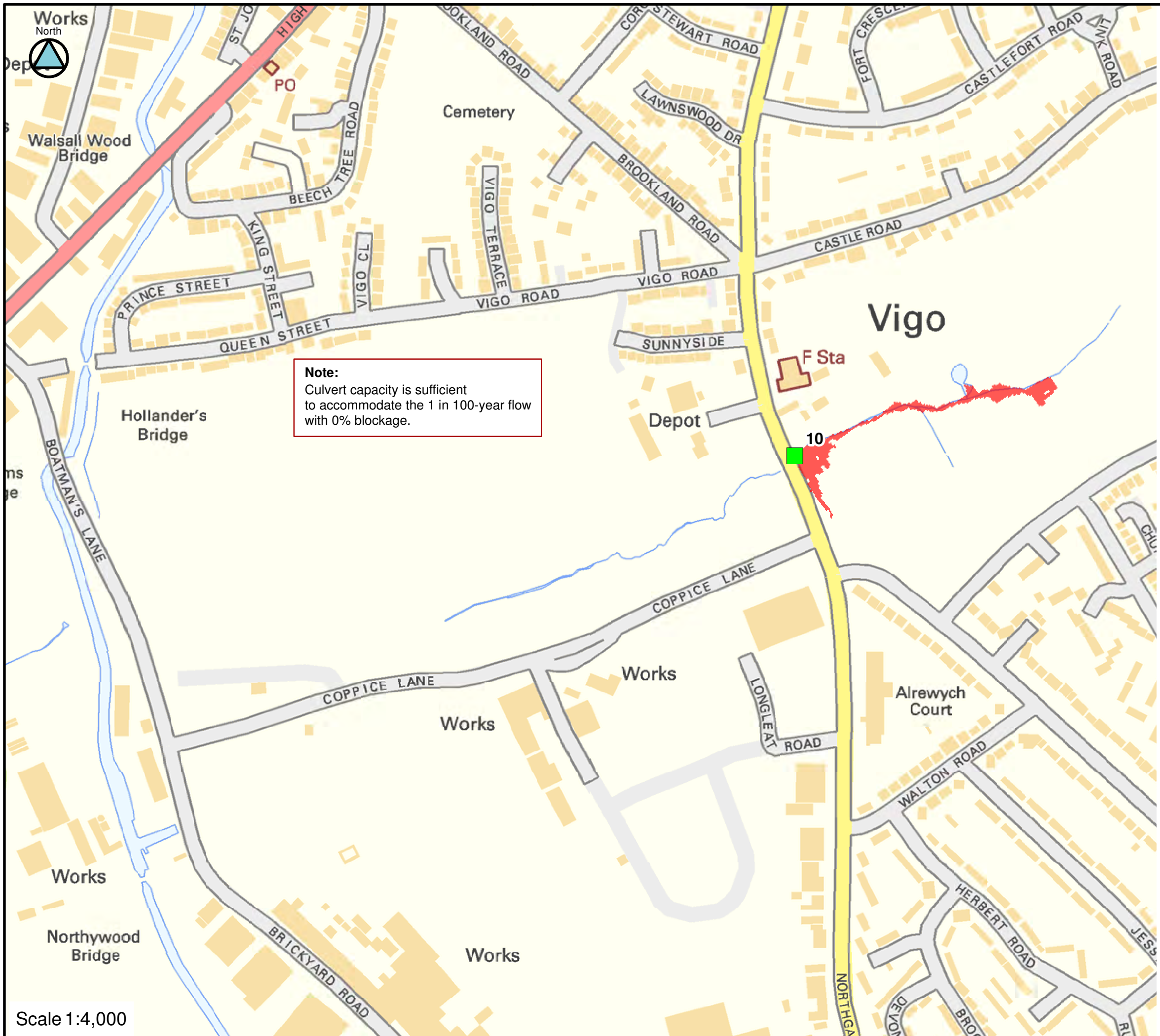
FIGURE C10-100-50 CULVERT 10 BLOCKAGE 1 IN 100-YEAR FLOOD EXTENTS
