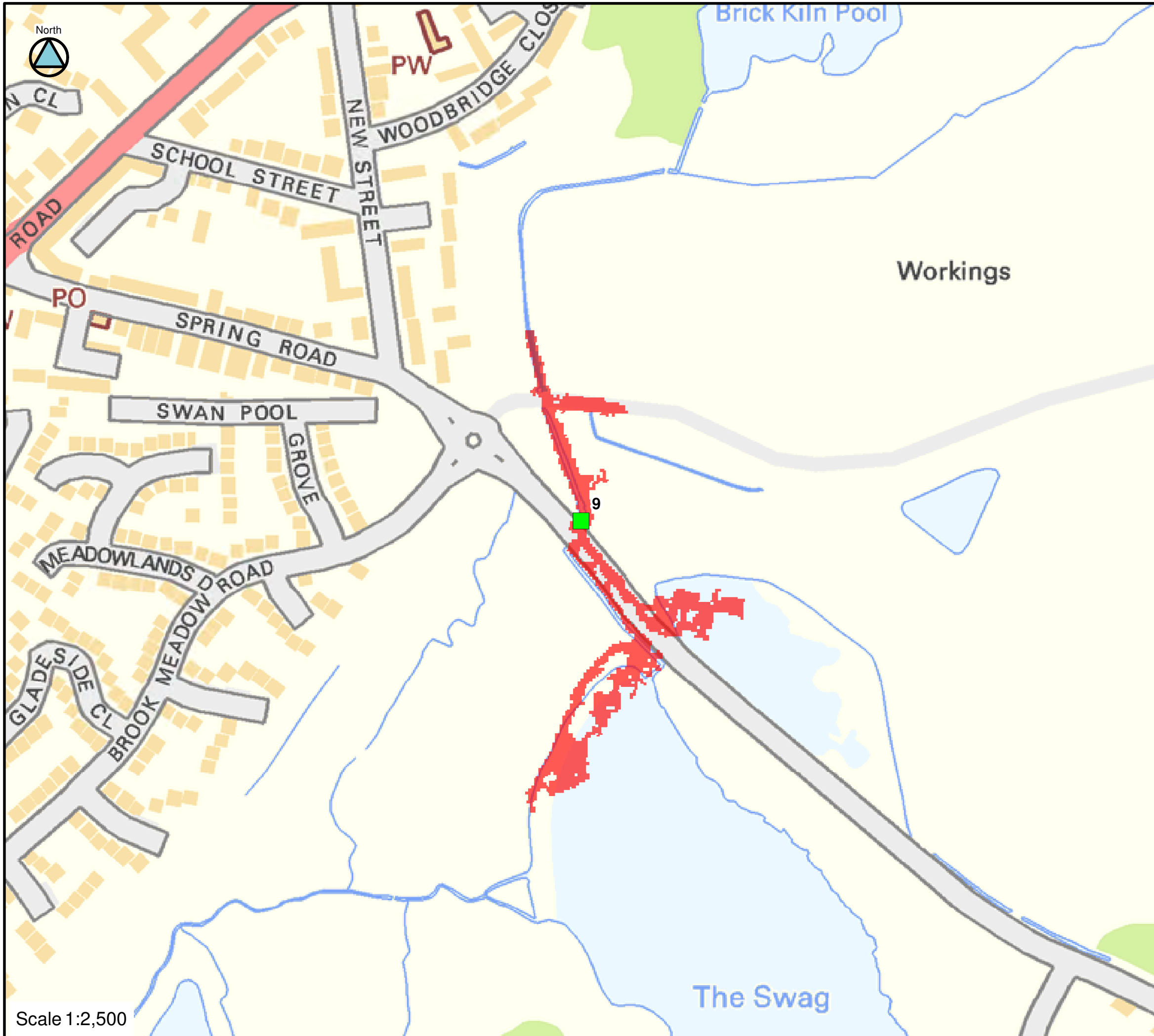
FIGURE C09-30-90 CULVERT 9 BLOCKAGE 1 IN 30-YEAR FLOOD EXTENTS
