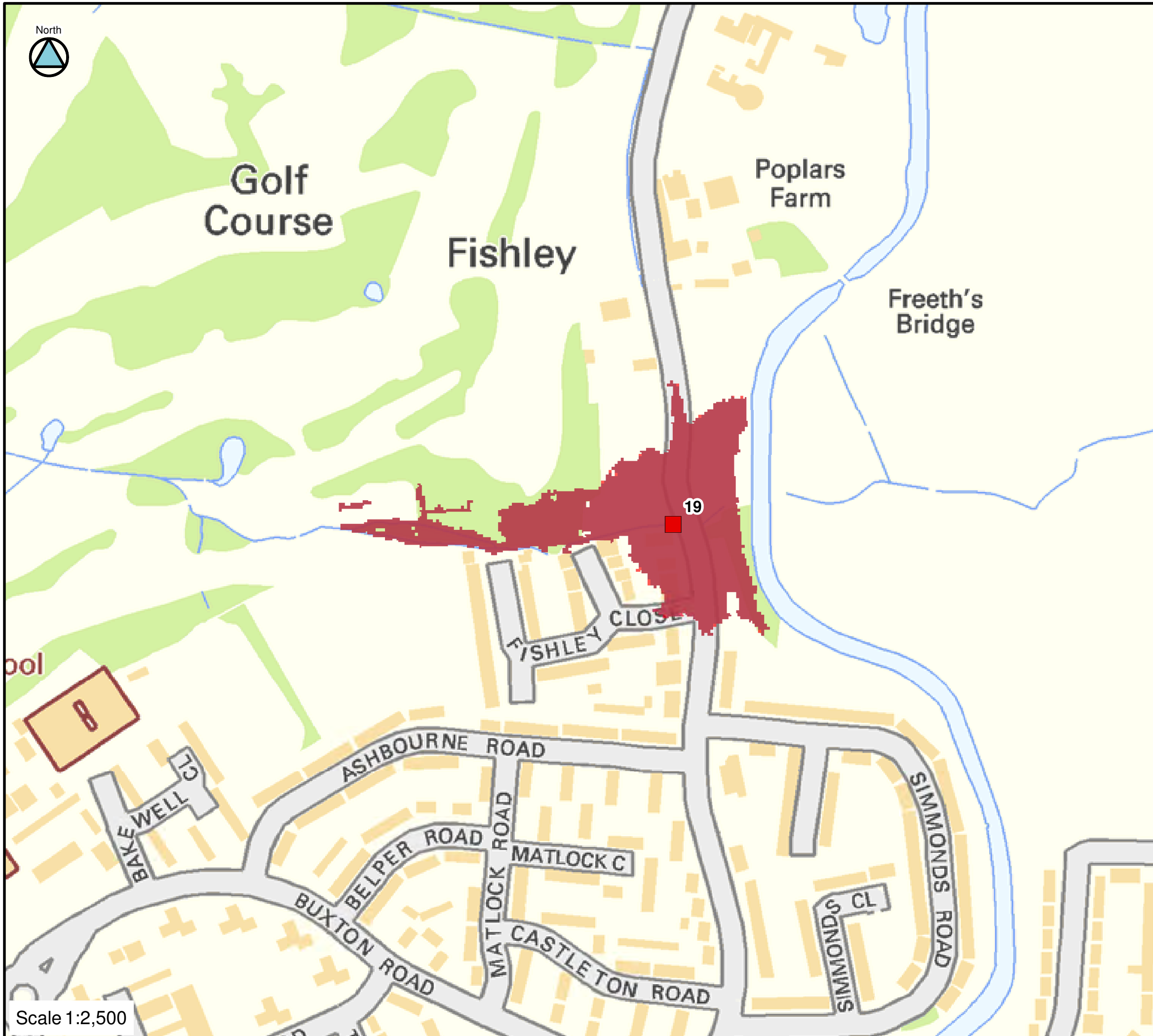
FIGURE C19-30-50 CULVERT 19 BLOCKAGE 1 IN 30-YEAR FLOOD EXTENTS
