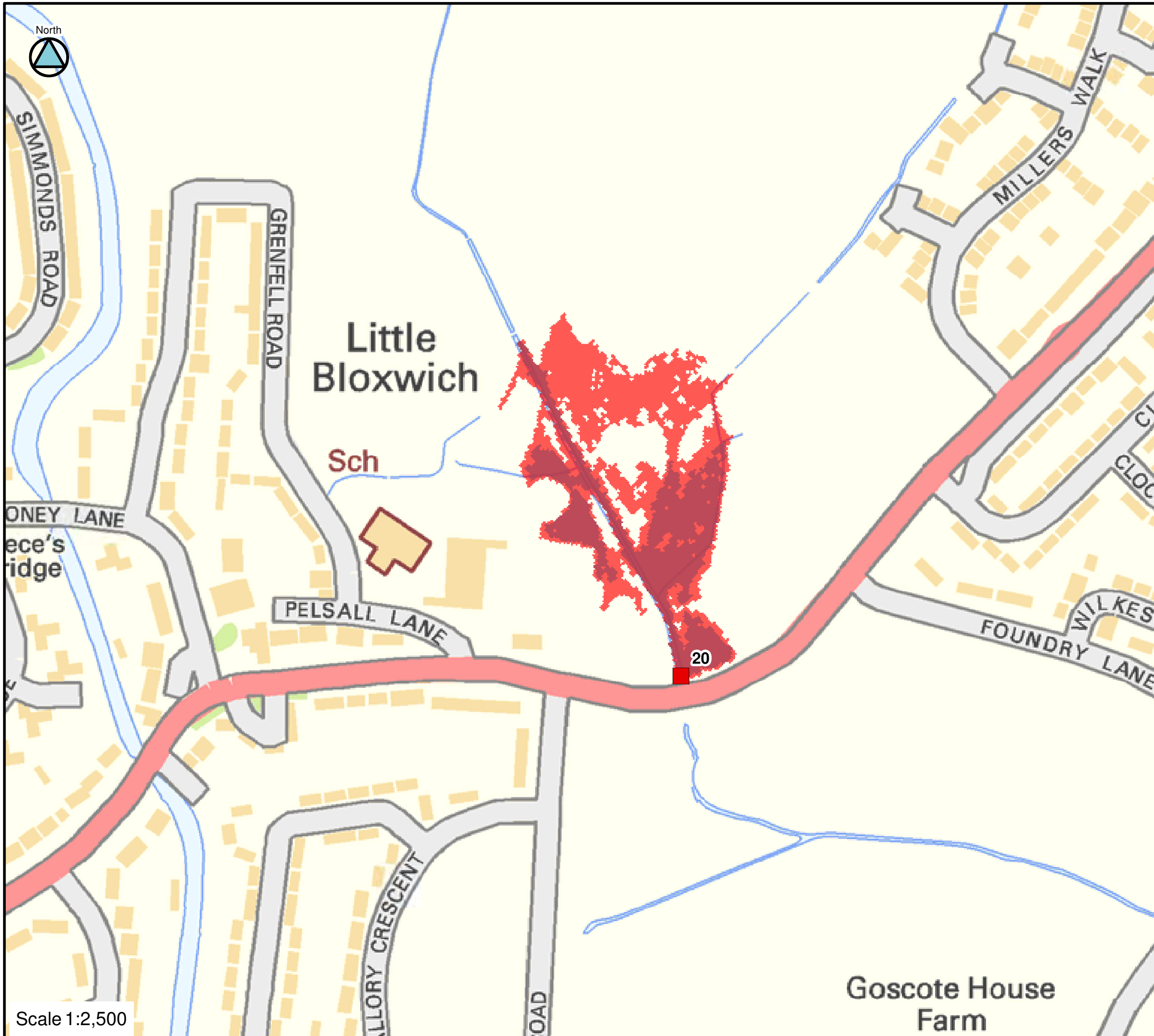
FIGURE C20-100-90 CULVERT 20 BLOCKAGE 1 IN 100-YEAR FLOOD EXTENTS
