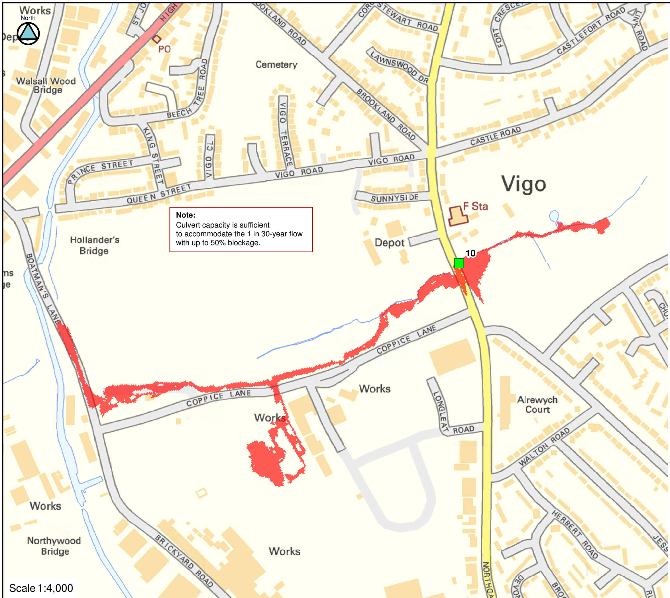
FIGURE C10-30-90 CULVERT 10 BLOCKAGE 1 IN 30-YEAR FLOOD EXTENTS
