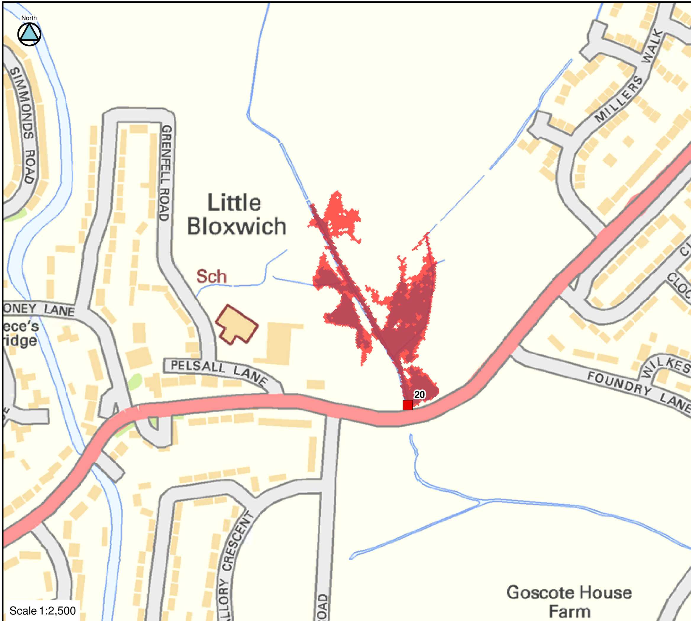
FIGURE C20-100-50 CULVERT 20 BLOCKAGE 1 IN 100-YEAR FLOOD EXTENTS
