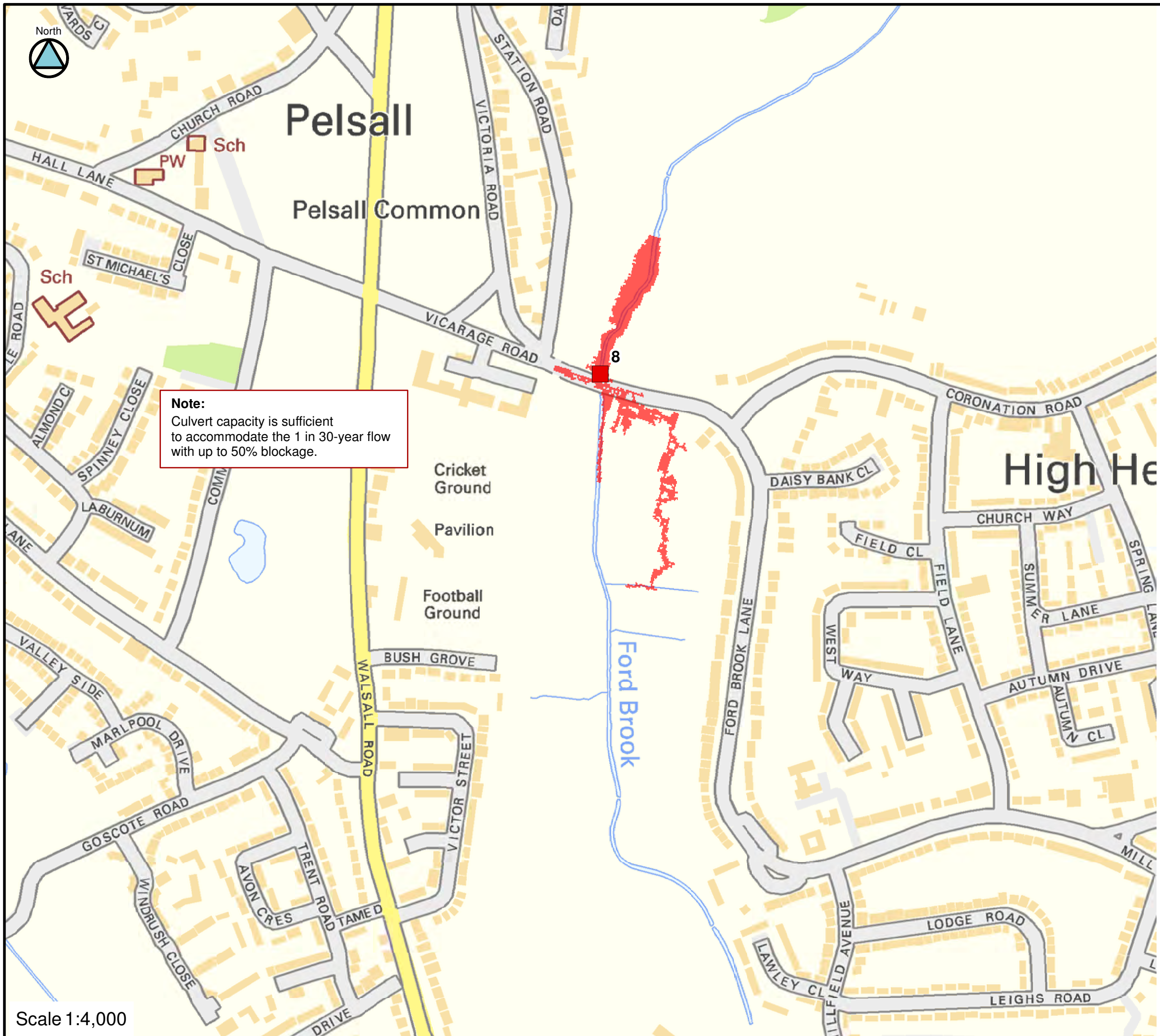
FIGURE C08-30-75 CULVERT 8 BLOCKAGE 1 IN 30-YEAR FLOOD EXTENTS
