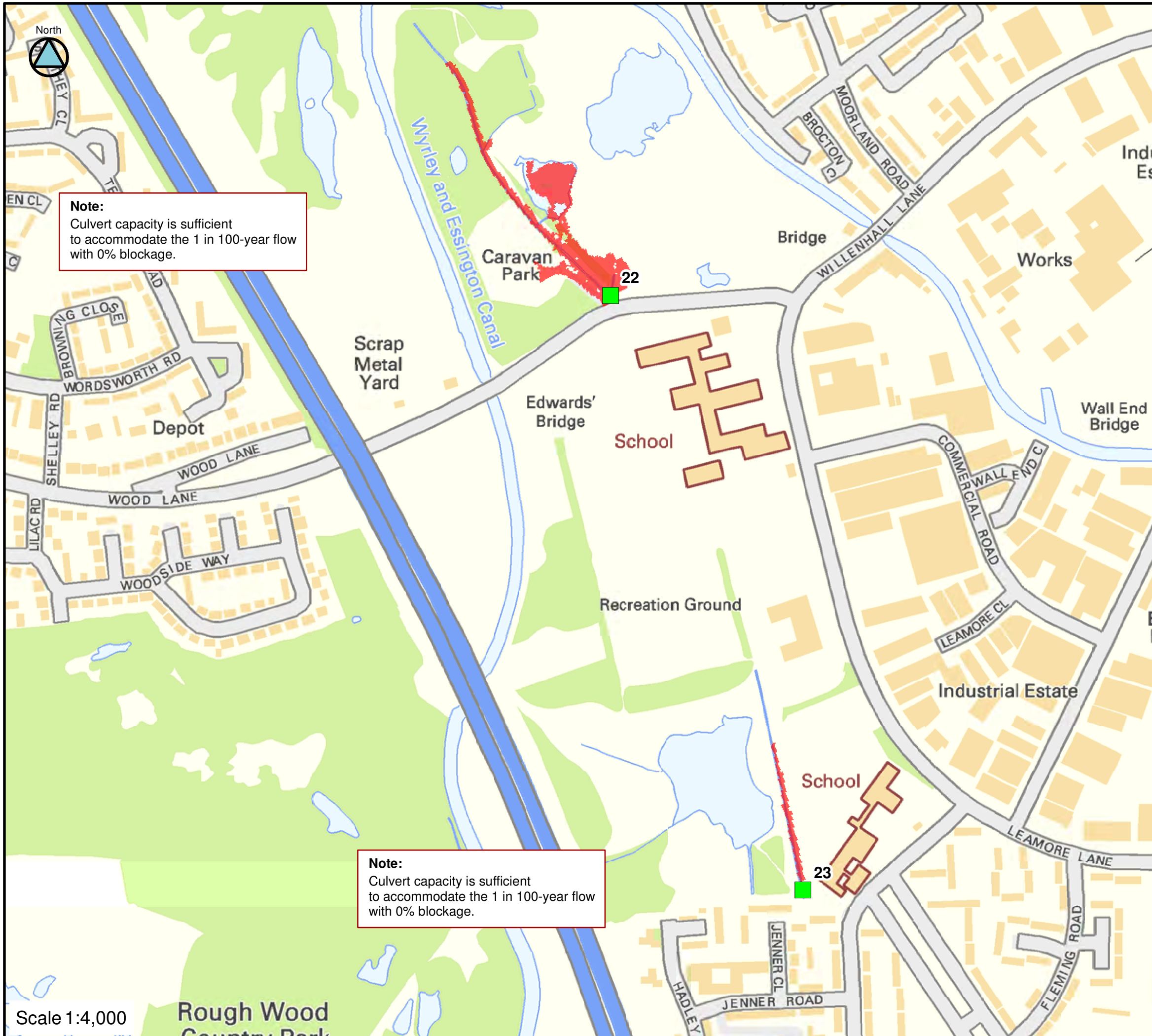
FIGURE C22-100-50 CULVERT 22&23 BLOCKAGE 1 IN 100-YEAR FLOOD EXTENTS
