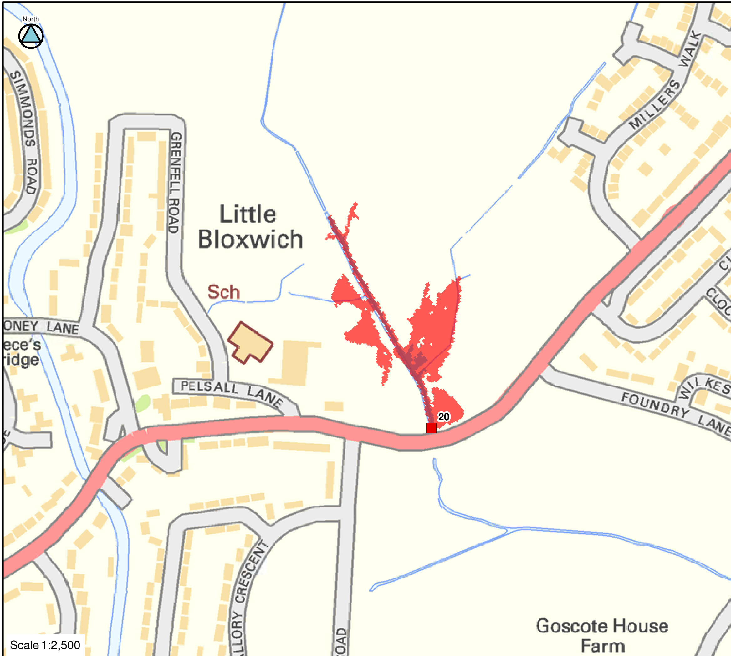
FIGURE C20-30-50 CULVERT 20 BLOCKAGE 1 IN 30-YEAR FLOOD EXTENTS
