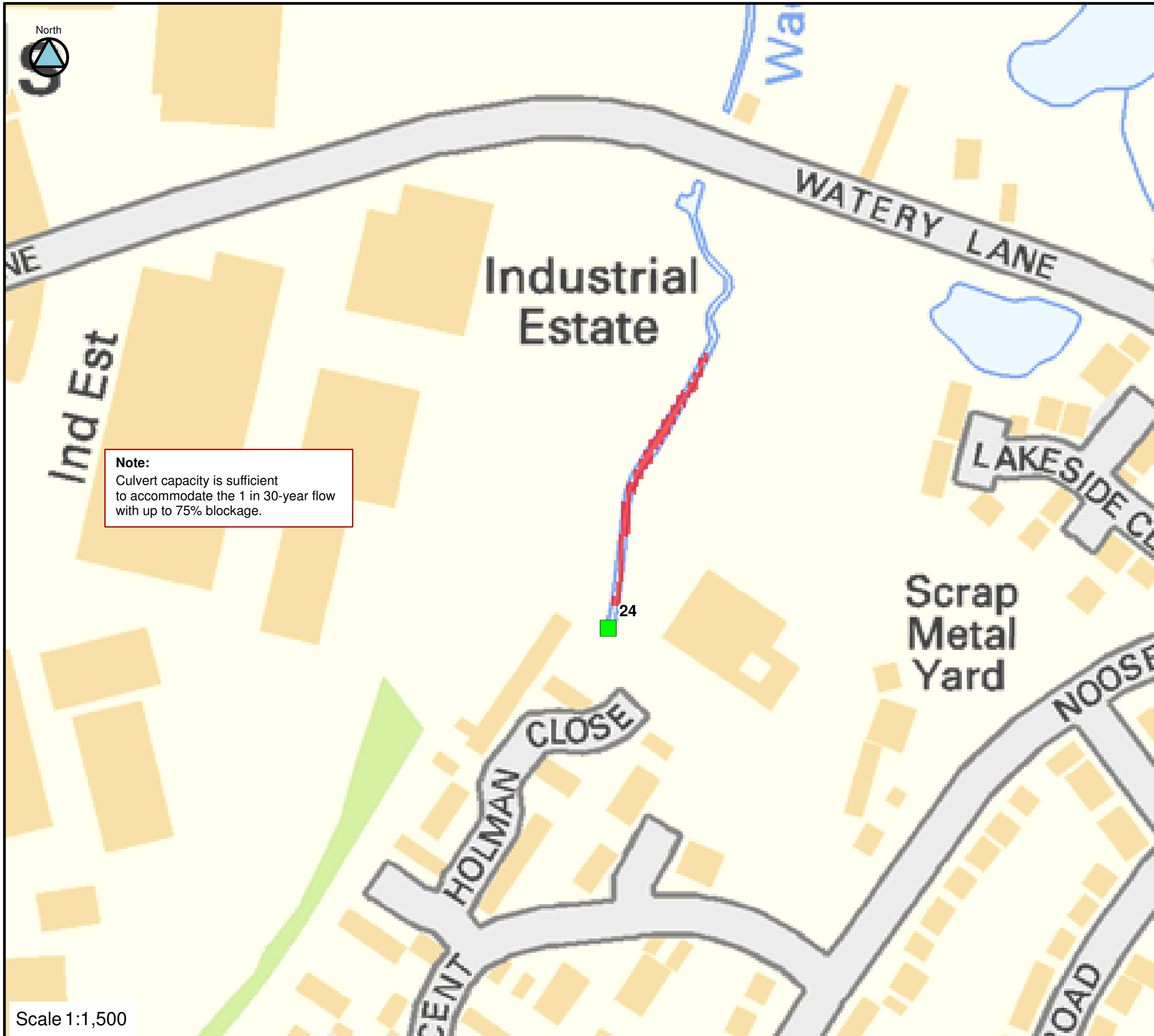
FIGURE C24-30-90 CULVERT 24 BLOCKAGE 1 IN 30-YEAR FLOOD EXTENTS
