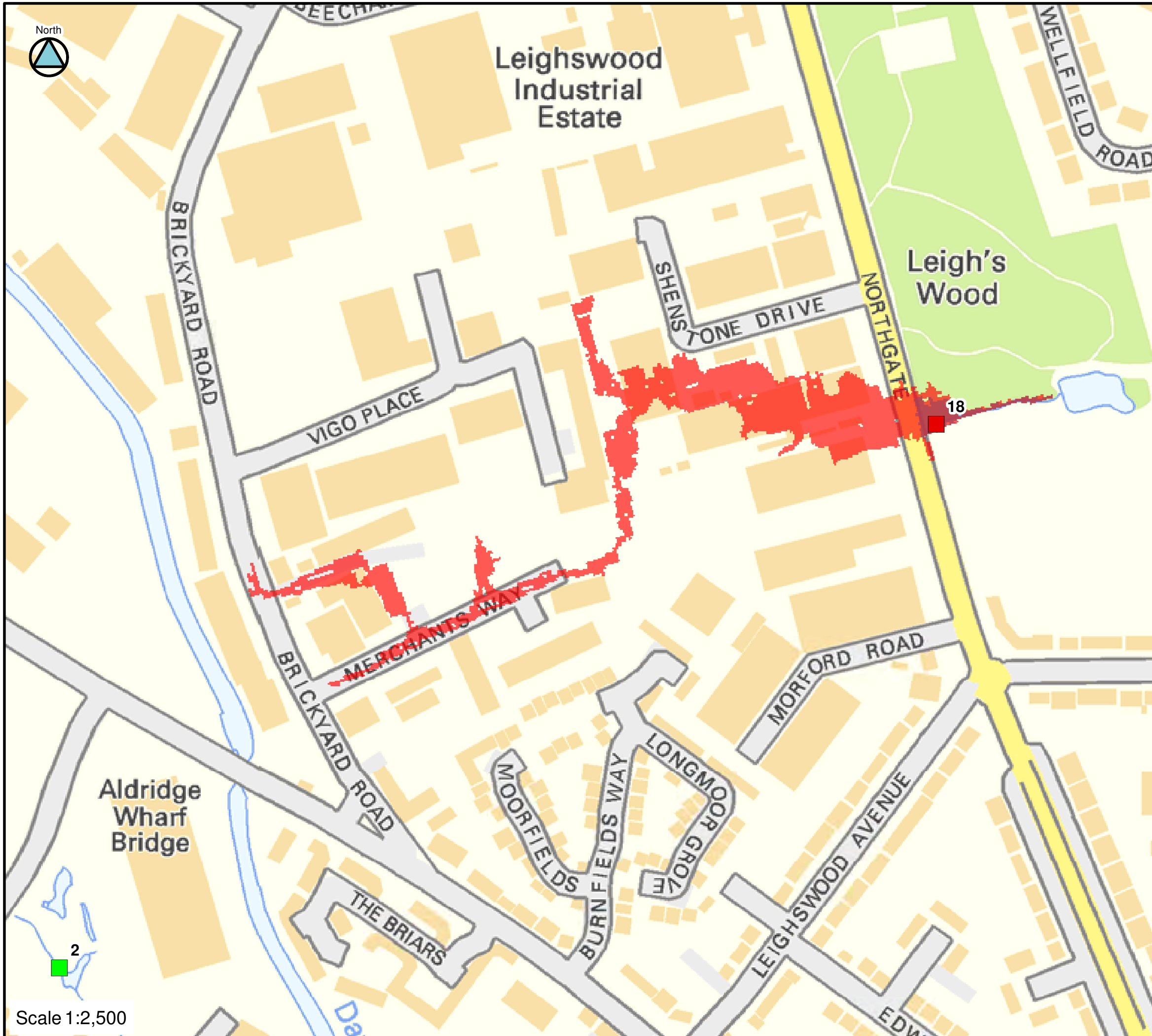
FIGURE C18-30-50 CULVERT 18 BLOCKAGE 1 IN 30-YEAR FLOOD EXTENTS
