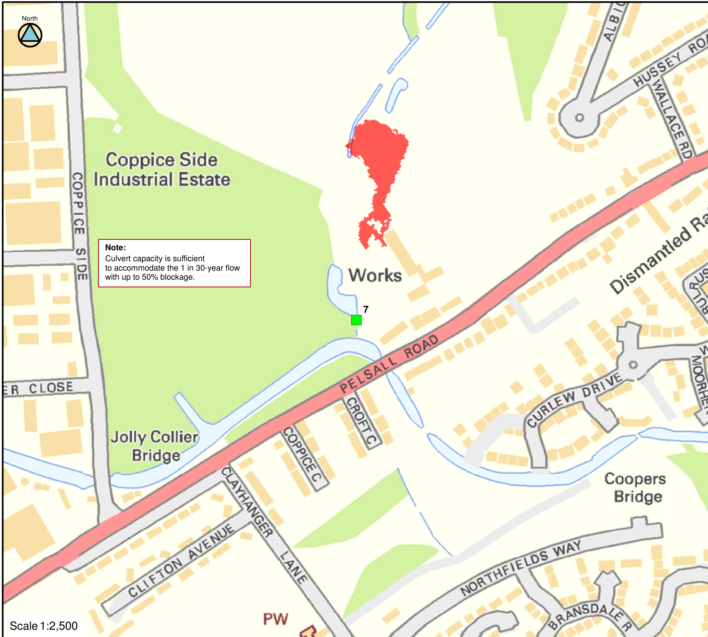
FIGURE C07-30-50 CULVERT 7 BLOCKAGE 1 IN 30-YEAR FLOOD EXTENTS
