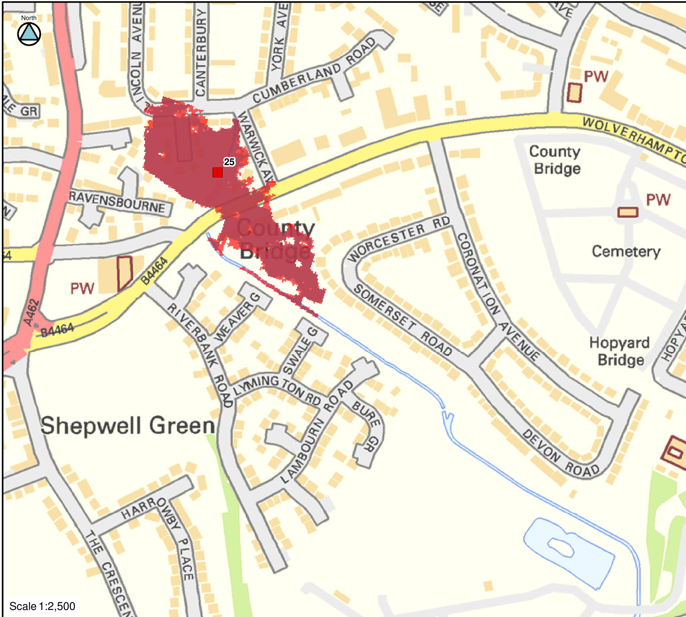
FIGURE C25-100-50 CULVERT 25 BLOCKAGE 1 IN 100-YEAR FLOOD EXTENTS
