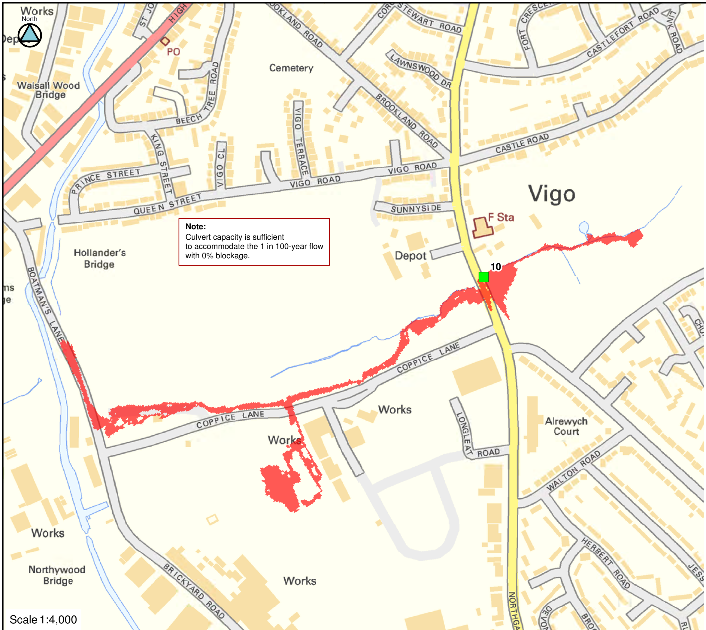
FIGURE C10-100-75 CULVERT 10 BLOCKAGE 1 IN 100-YEAR FLOOD EXTENTS
