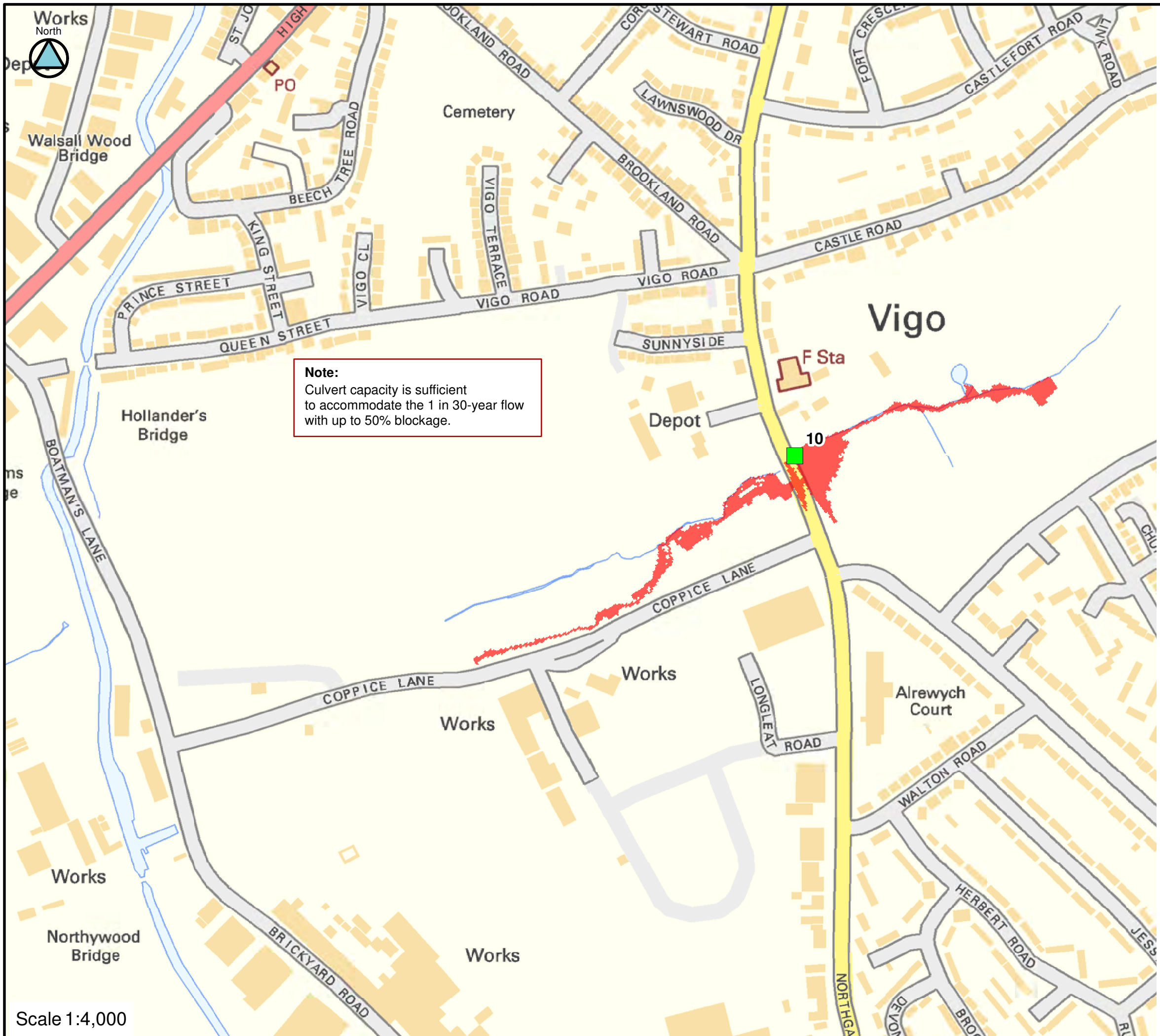
FIGURE C10-30-75 CULVERT 10 BLOCKAGE 1 IN 30-YEAR FLOOD EXTENTS
