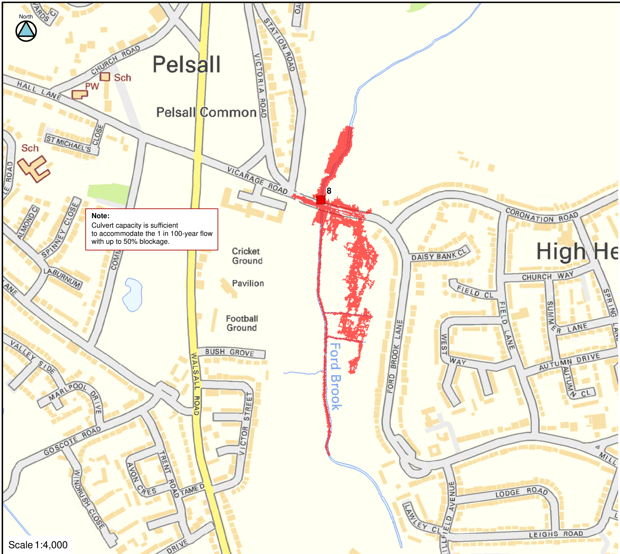
FIGURE C08-100-75 CULVERT 8 BLOCKAGE 1 IN 100-YEAR FLOOD EXTENTS
