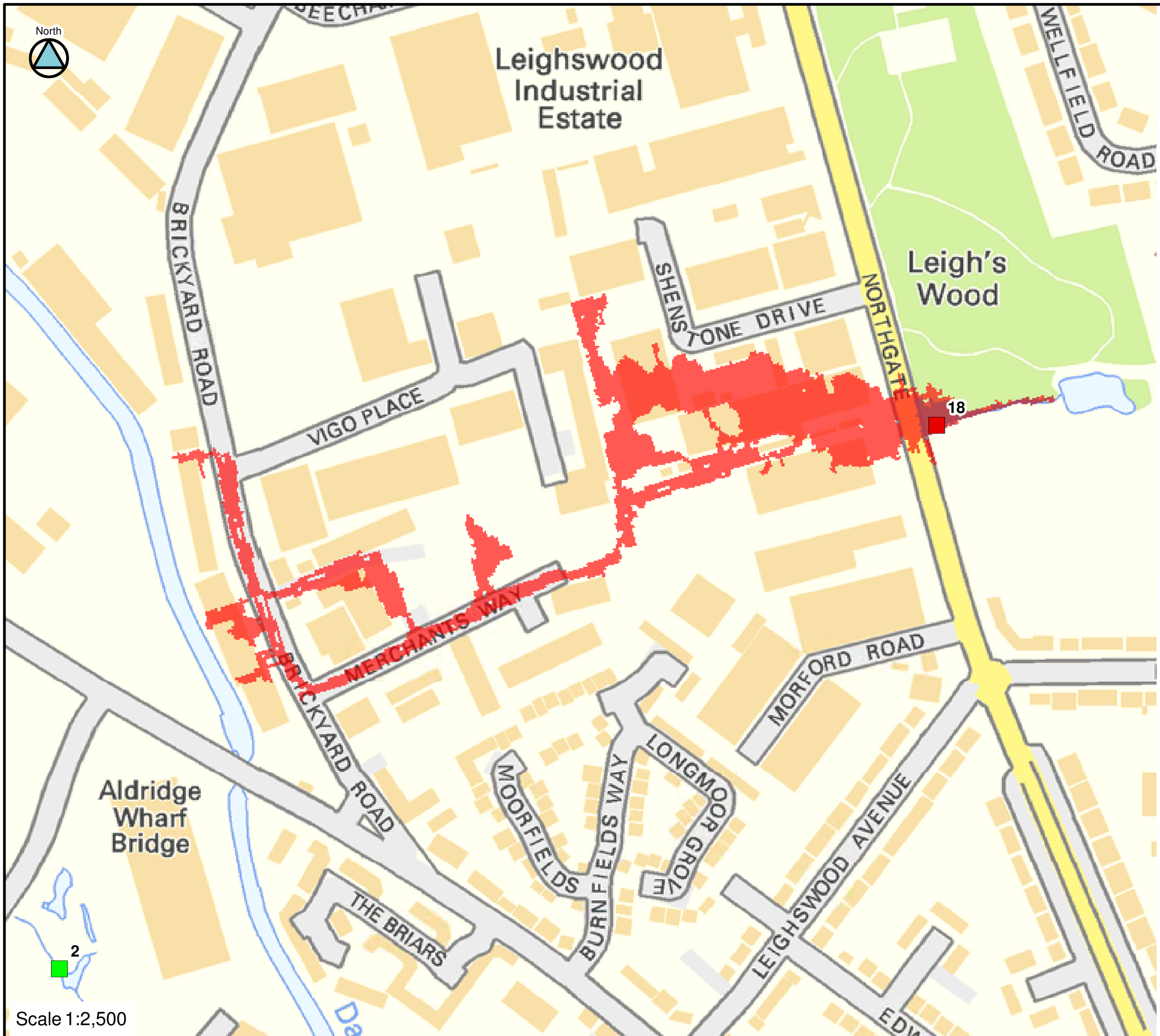
FIGURE C18-30-75 CULVERT 18 BLOCKAGE 1 IN 30-YEAR FLOOD EXTENTS
