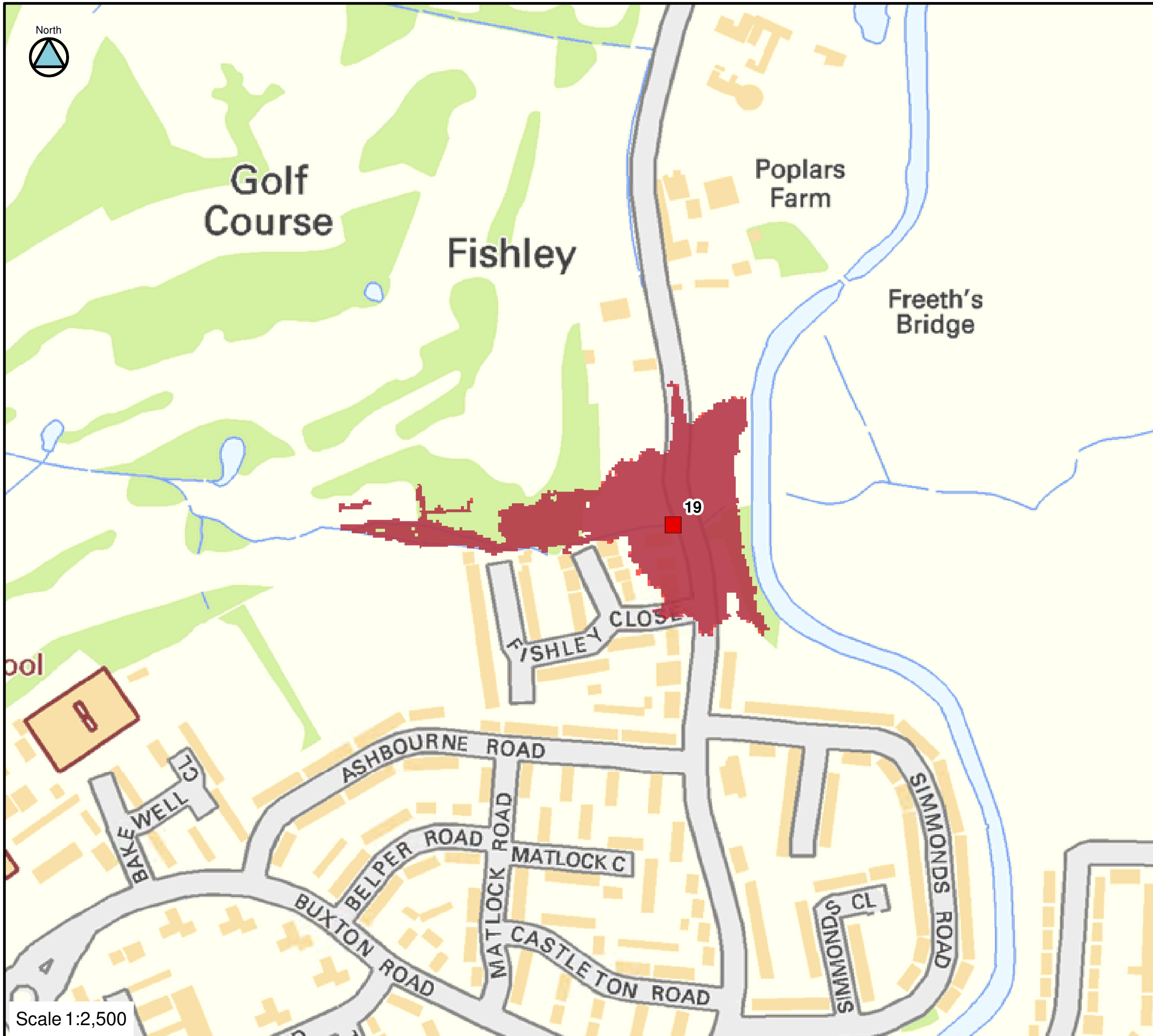
FIGURE C19-30-90 CULVERT 19 BLOCKAGE 1 IN 30-YEAR FLOOD EXTENTS
