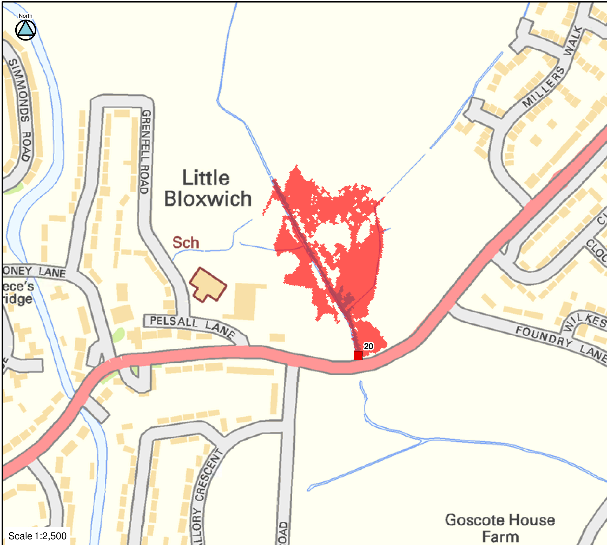
FIGURE C20-30-90 CULVERT 20 BLOCKAGE 1 IN 30-YEAR FLOOD EXTENTS
