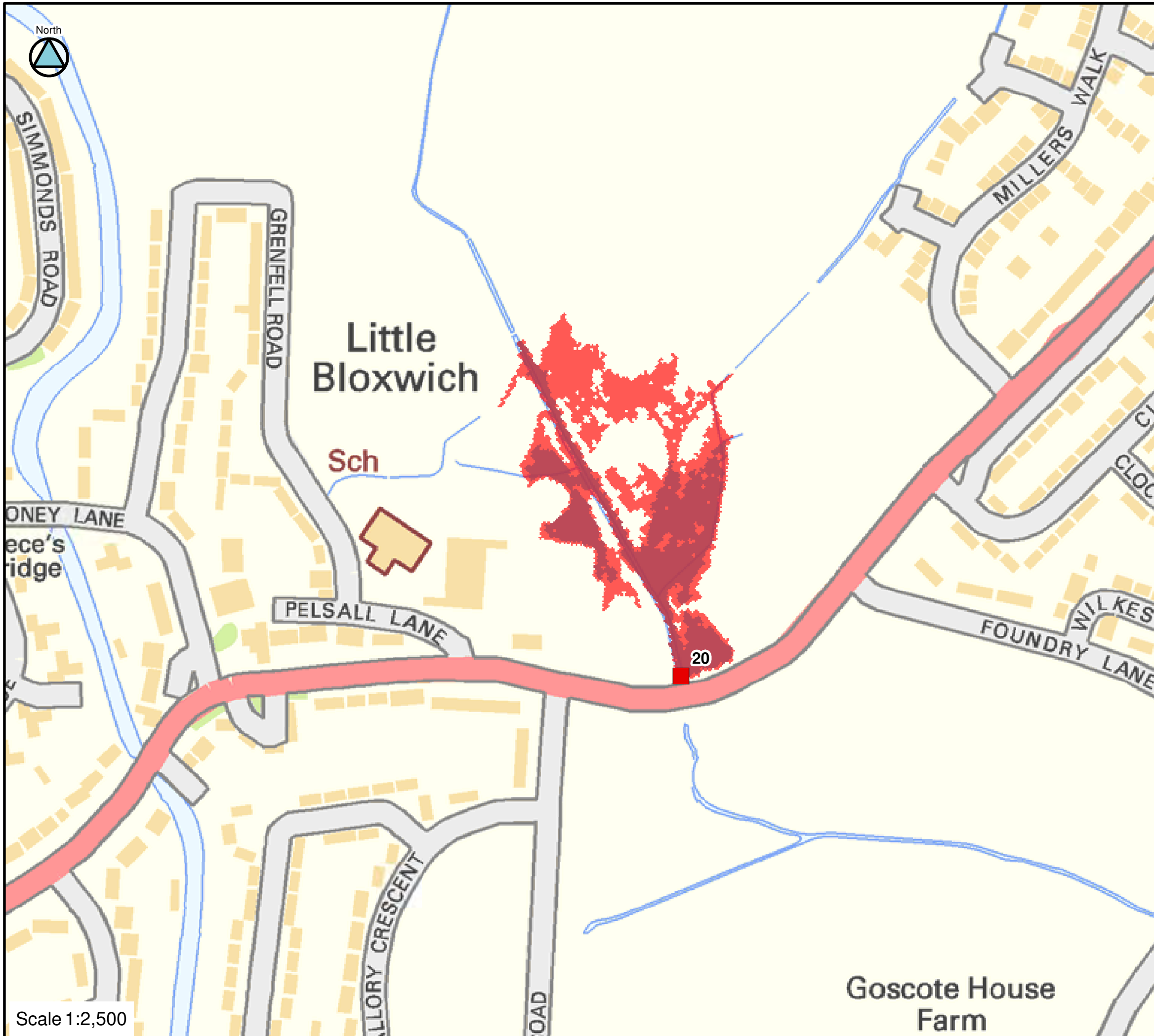
FIGURE C20-100-75 CULVERT 20 BLOCKAGE 1 IN 100-YEAR FLOOD EXTENTS
