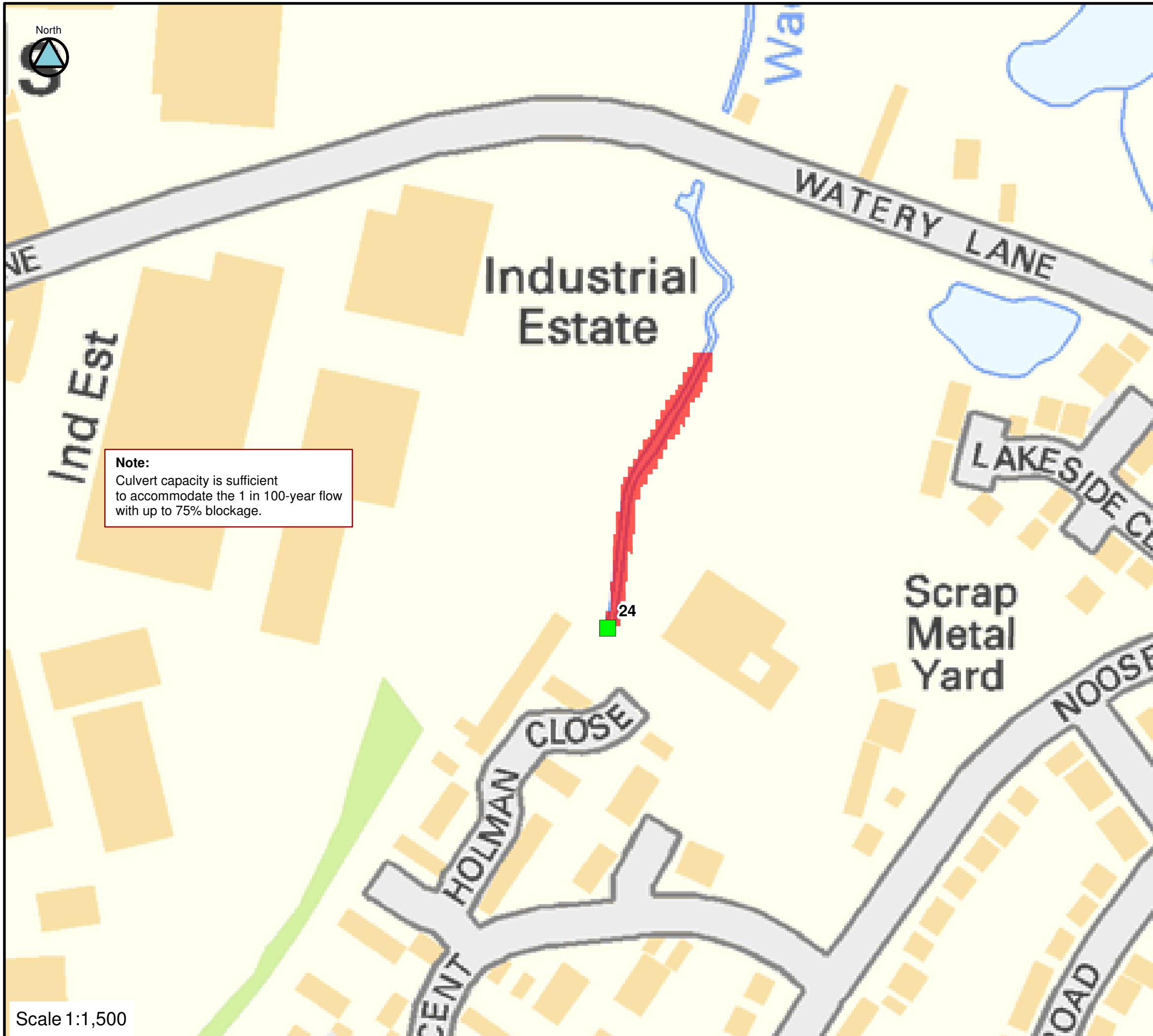
FIGURE C24-100-90 CULVERT 24 BLOCKAGE 1 IN 100-YEAR FLOOD EXTENTS
