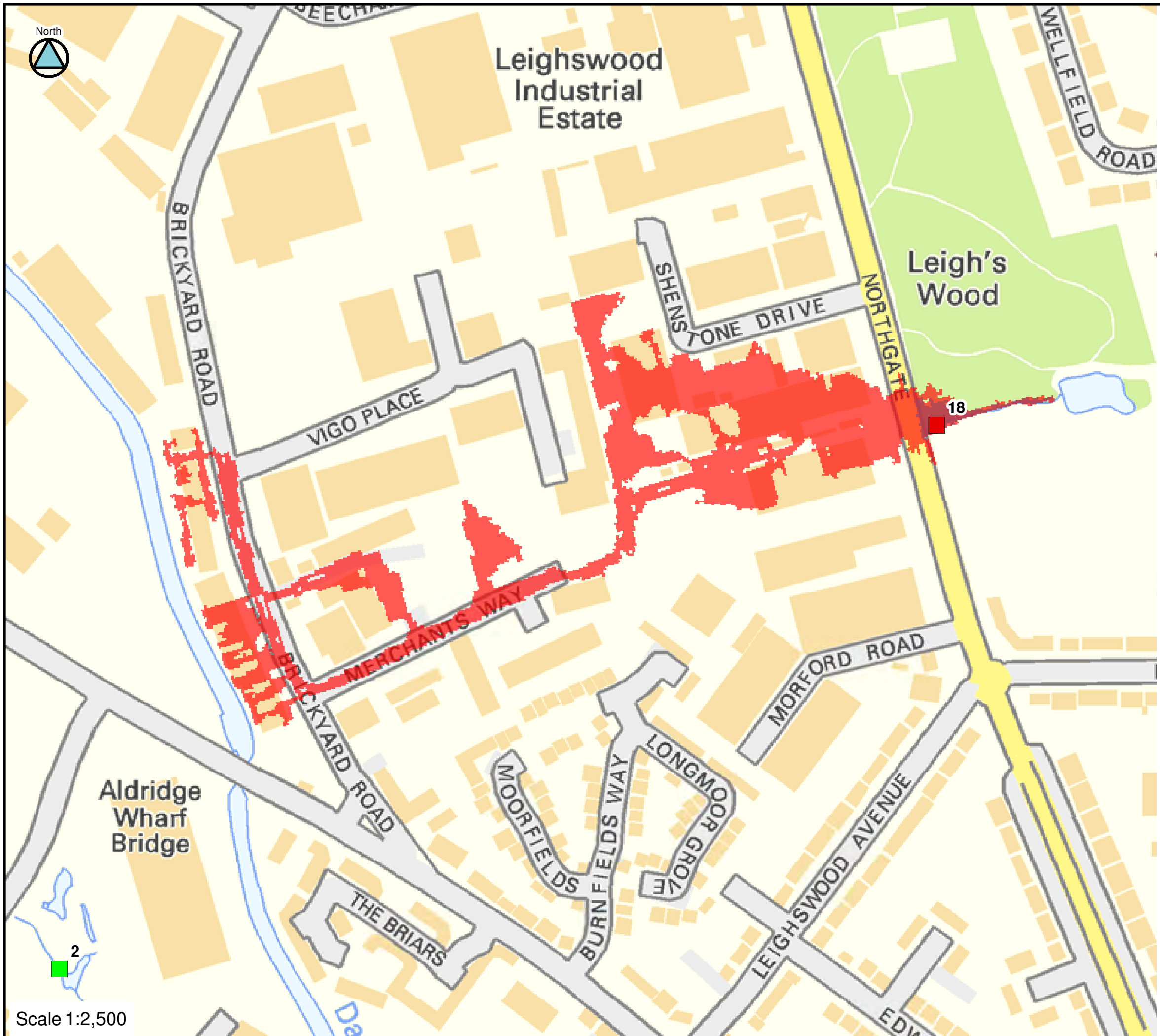
FIGURE C18-30-90 CULVERT 18 BLOCKAGE 1 IN 30-YEAR FLOOD EXTENTS
