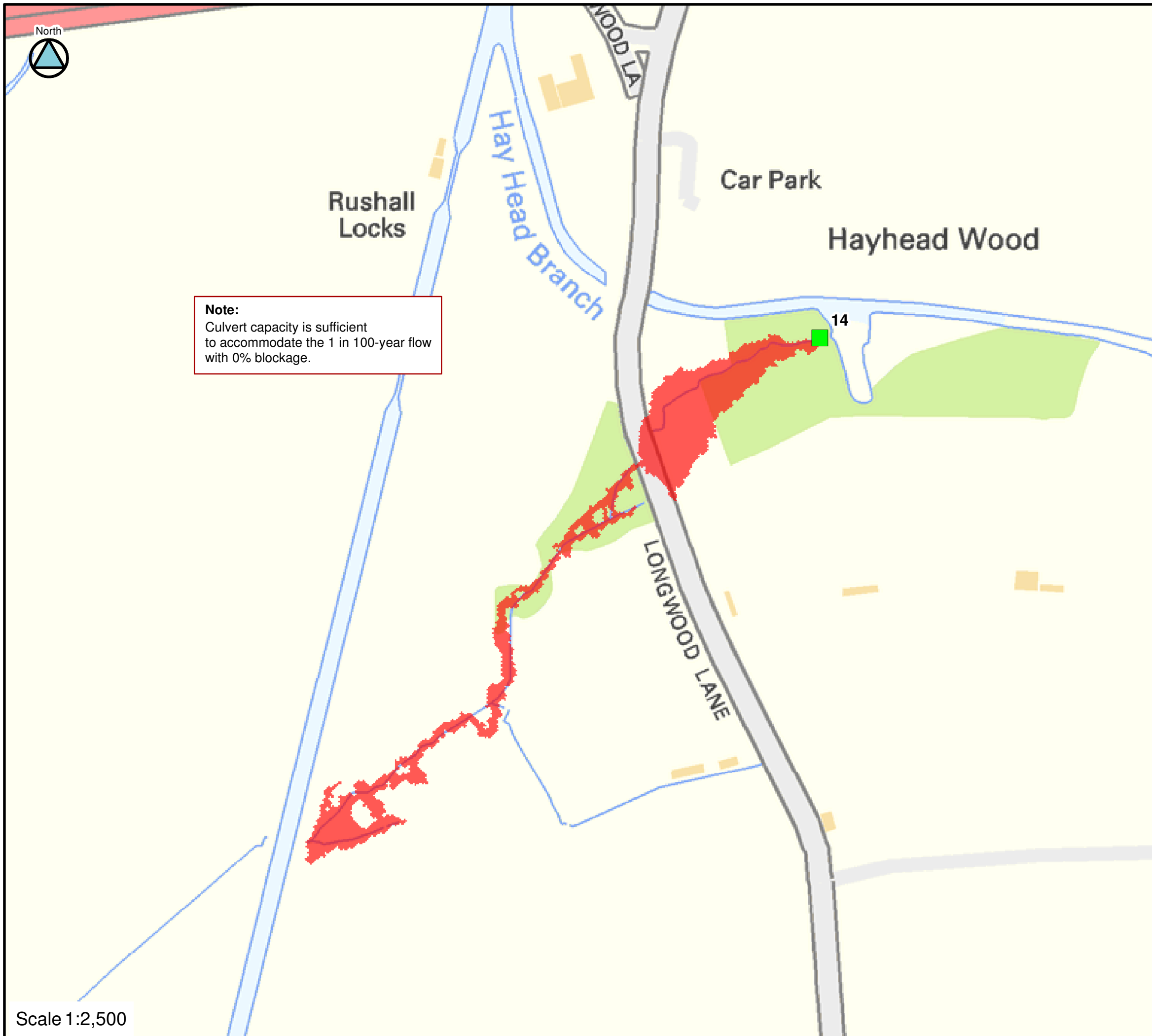
FIGURE C14-100-75 CULVERT 14 BLOCKAGE 1 IN 100-YEAR FLOOD EXTENTS
