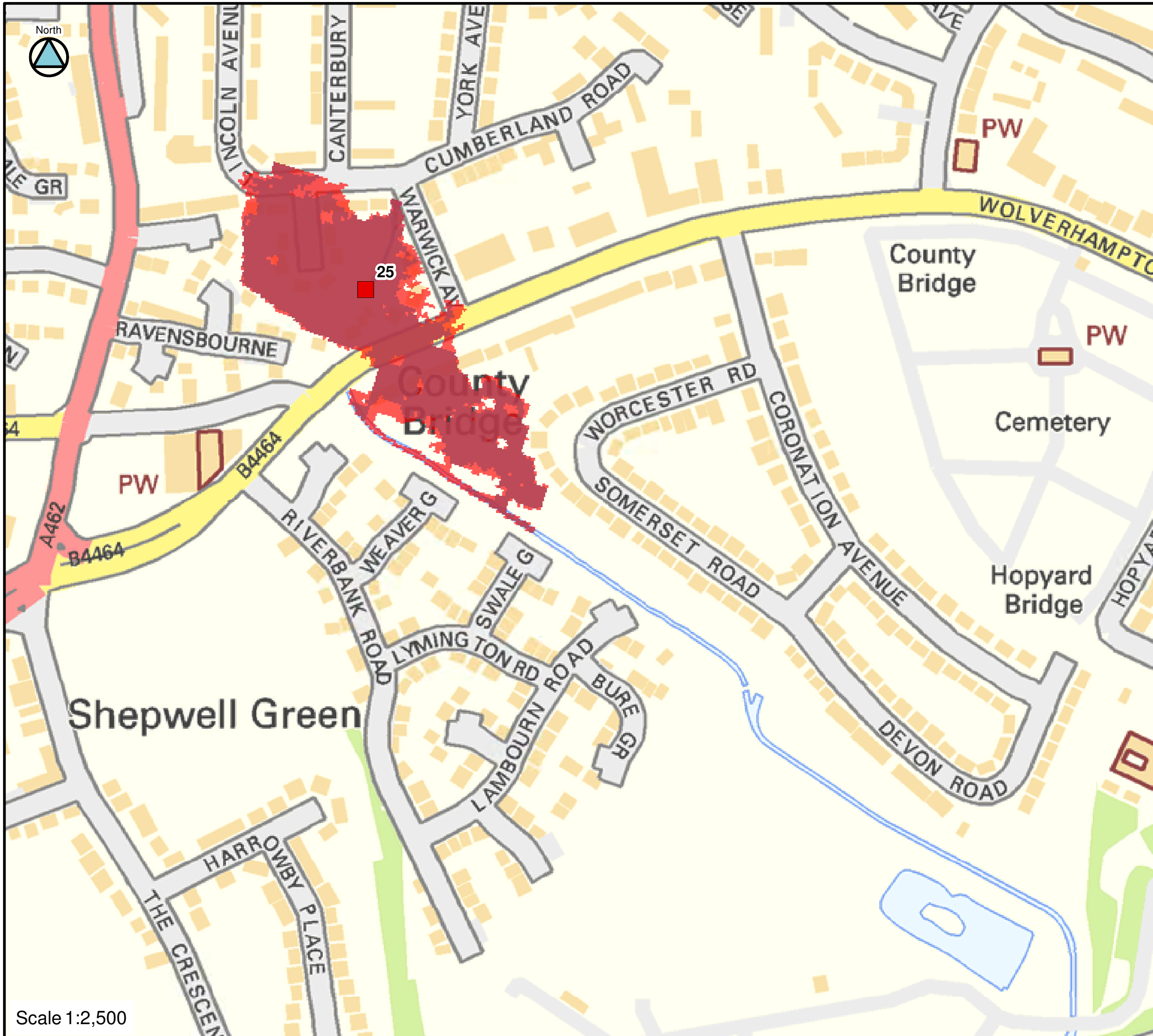
FIGURE C25-100-90 CULVERT 25 BLOCKAGE 1 IN 100-YEAR FLOOD EXTENTS
