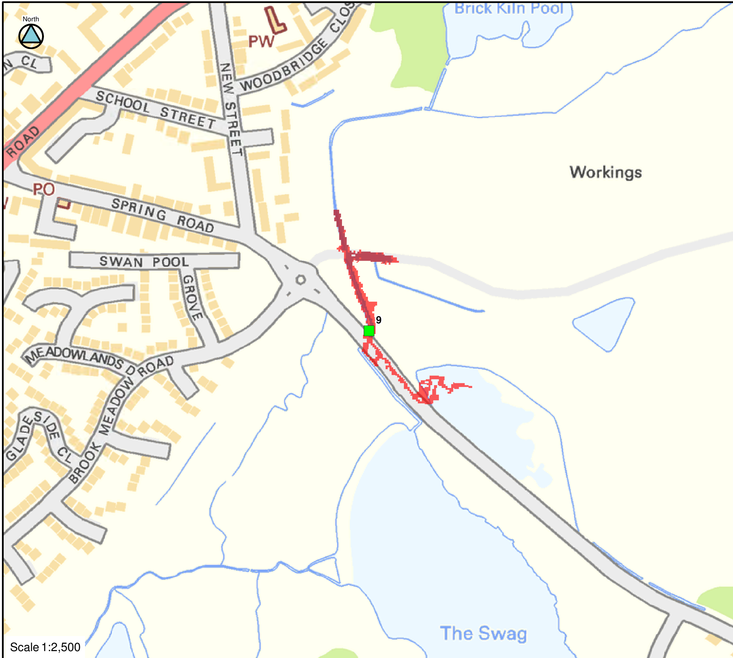
FIGURE C09-100-50 CULVERT 9 BLOCKAGE 1 IN 100-YEAR FLOOD EXTENTS
