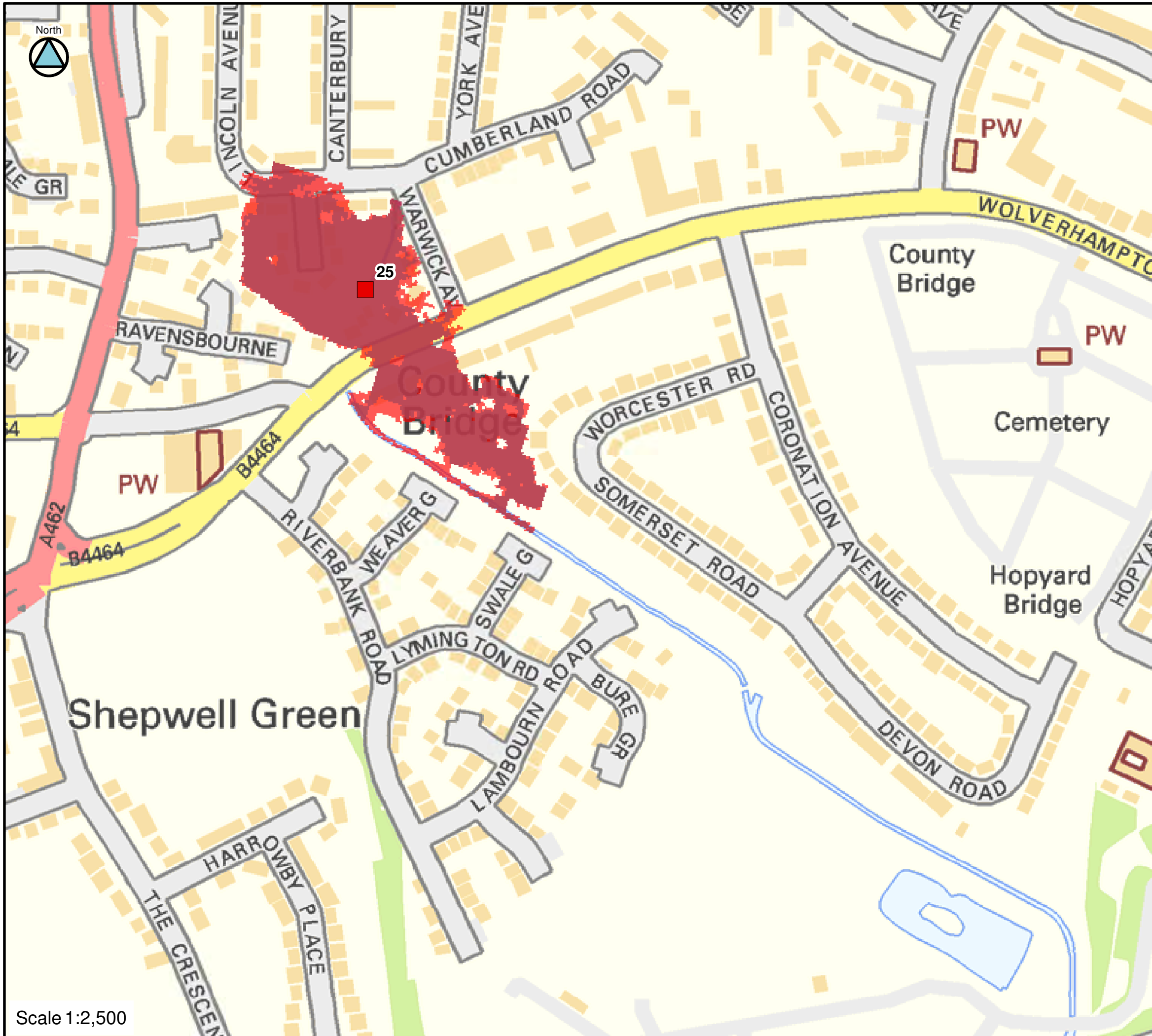
FIGURE C25-100-75 CULVERT 25 BLOCKAGE 1 IN 100-YEAR FLOOD EXTENTS
