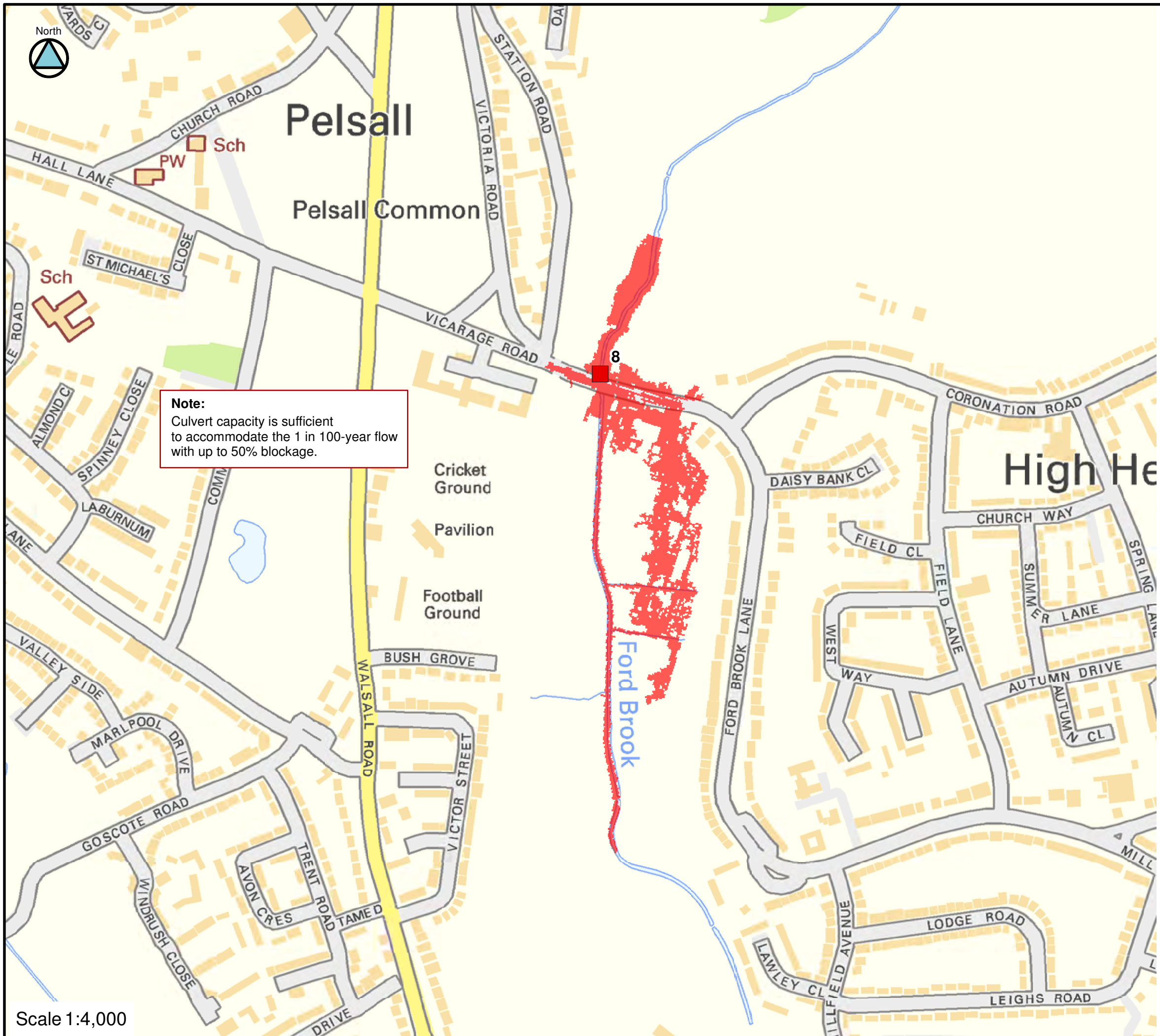
FIGURE C08-100-90 CULVERT 8 BLOCKAGE 1 IN 100-YEAR FLOOD EXTENTS
