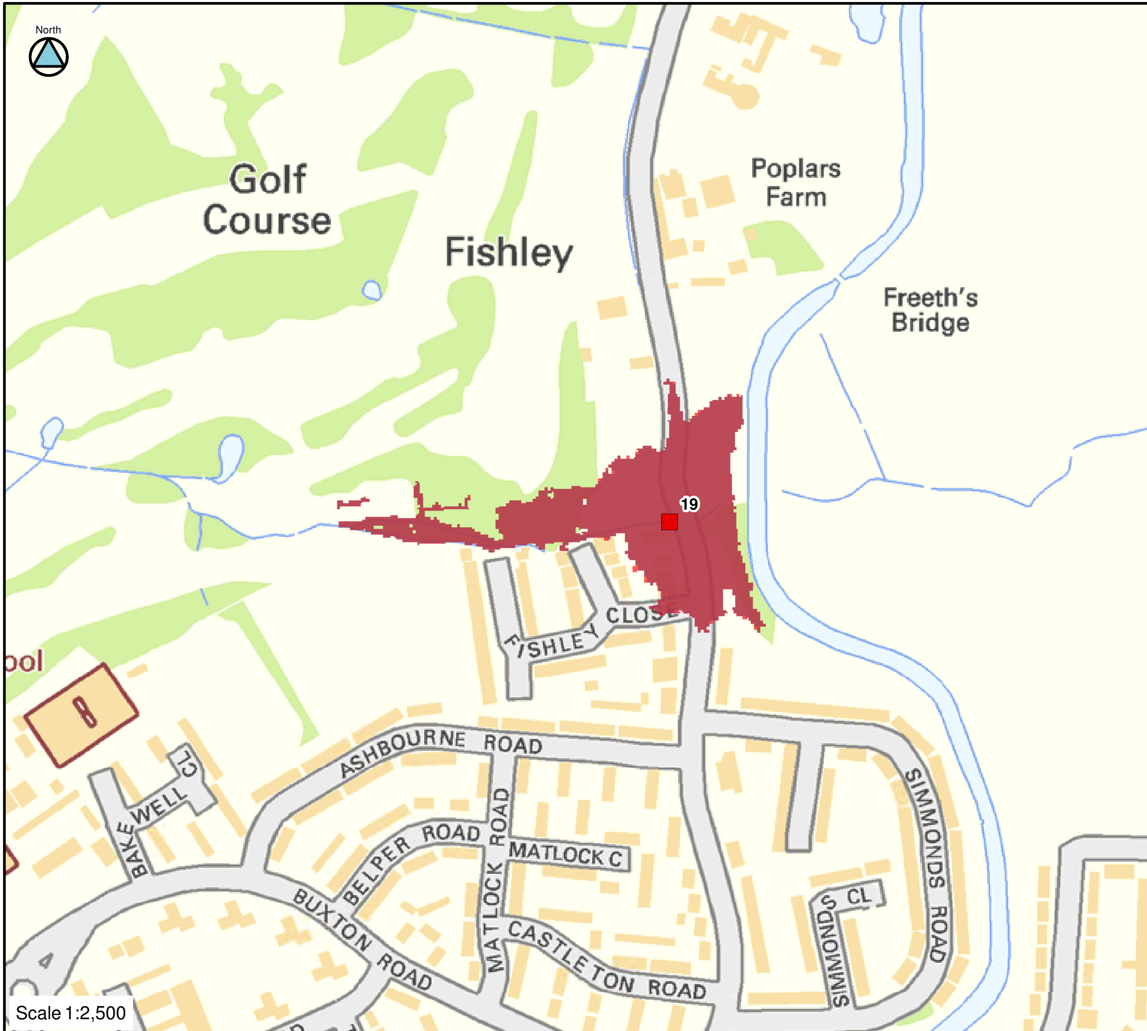
FIGURE C19-30-75 CULVERT 19 BLOCKAGE 1 IN 30-YEAR FLOOD EXTENTS
